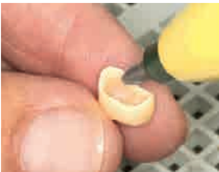
Lab: Sandblast the bonding surface with alumina, 50 µm grain size at 2 bars (30 PSI).
